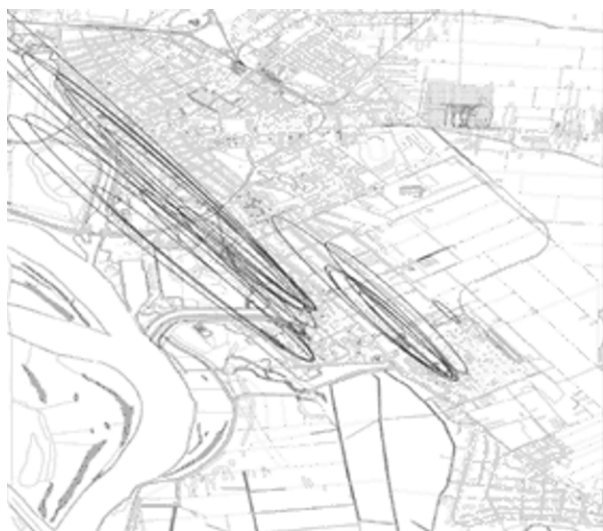
Fig. 2. Cumulative effect of dispersion of NO 2 in the oil and petrochemical complex for the emission values.
